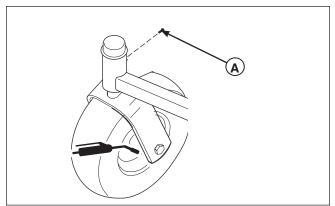
Figure 22. Front Caster & Wheel A. 1/4-28 Bolt
